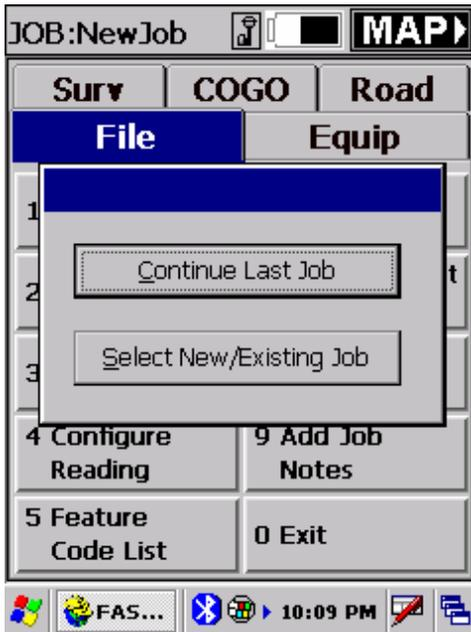
N. Although data from the Z-Max is coming into the MMCE's COM4 port along Bluetooth Channel 1 (in this example), this data must now be directed to FAST Survey. Tap the **Equip** tab and tap Option 8 (**Comm Setup**)
